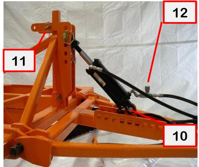
12. Hydraulic flow valves are standard, the front cylinder regulated going down, pan cylinders are regulated up & down!
