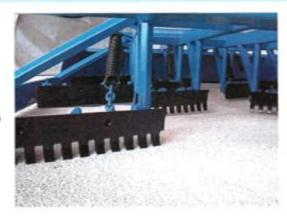
The standard serrated cutting blades are very effective in those hard icy trail conditions. Blade support struts have been rotated 45 degrees to promote the free flow of snow through the drag.
