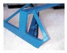
Front "nose cones" are reinforced to cut through hard packed snow. Tree guards and shear pin hitches eliminate the "oops" when cornering.
