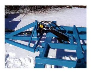
All Mogul Masters incorporate a unique floating device on the hitch to reduce scalping when cresting a hill. The chain hooks on the hitch make the connection to the track vehicle a simple, one man job that takes only minutes.
